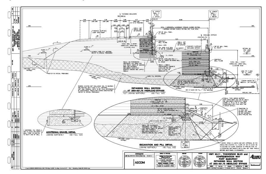
Figure 8 – Thickwood Boulevard Interchange Cross-section
