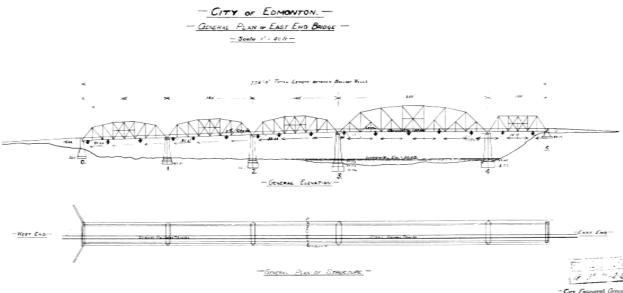
Figure 1: Original general arrangement drawing of Dawson Bridge.
