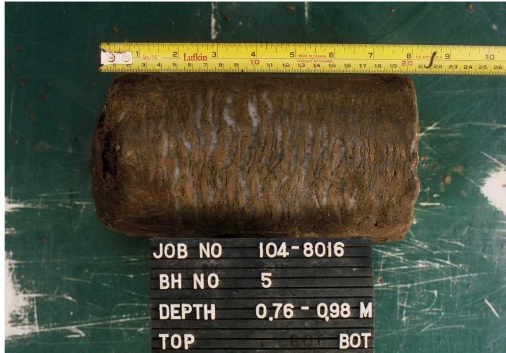
Photo 1: Ice Lenses in a Core of Frozen Silt Showing Frost Heave Mechanism
