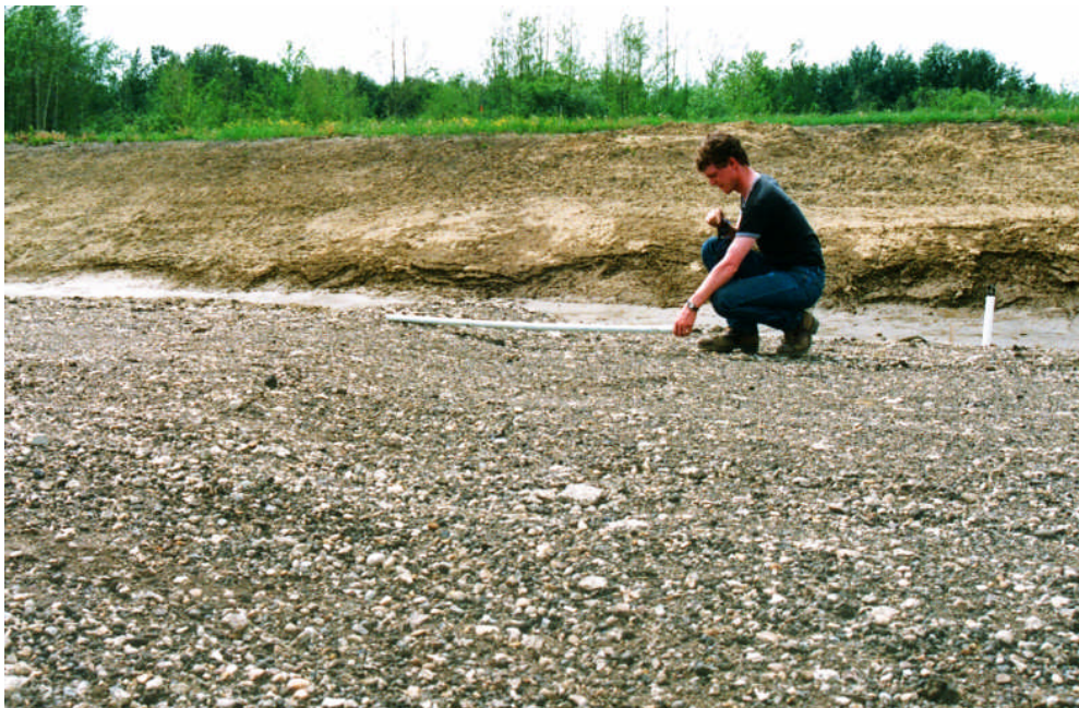
Photo 4: Frost Heave of 200 mm
