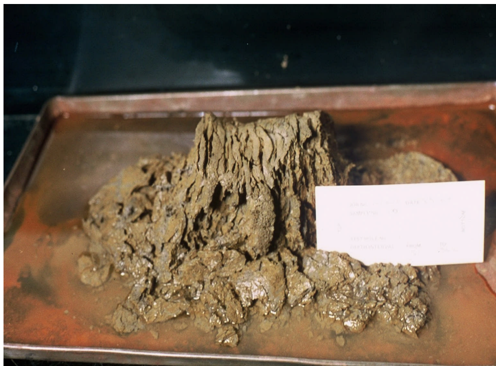
Photo 2: Loss of Strength upon Thawing
