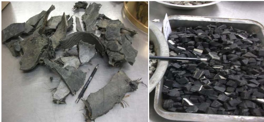
**Figure 1. Shredded Tires in Raw State (left) and Cut Into Smaller Pieces (right).**
