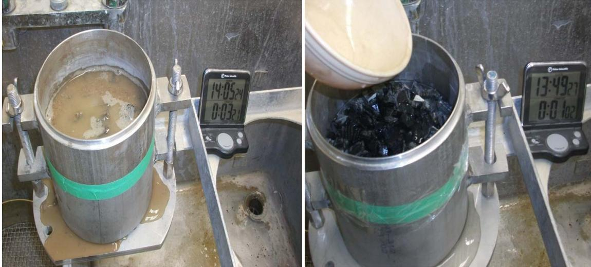
**Figure 6. Free Drainage Test.**
