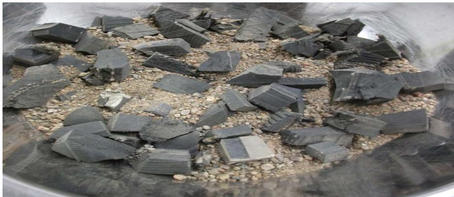
**Figure 2. Shredded tire/sand in the mix ratio of 1:2.**
