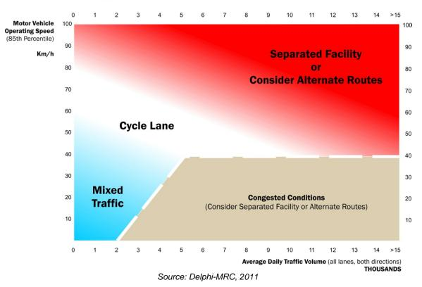
It is clear from the nomograph above that the decision to provide a segregated cycle facility is not binary. The nomograph actually provides guidance to practitioners on the potential application of other facility types such as cycle lanes, shared facilities and the consideration of alternative routes.
