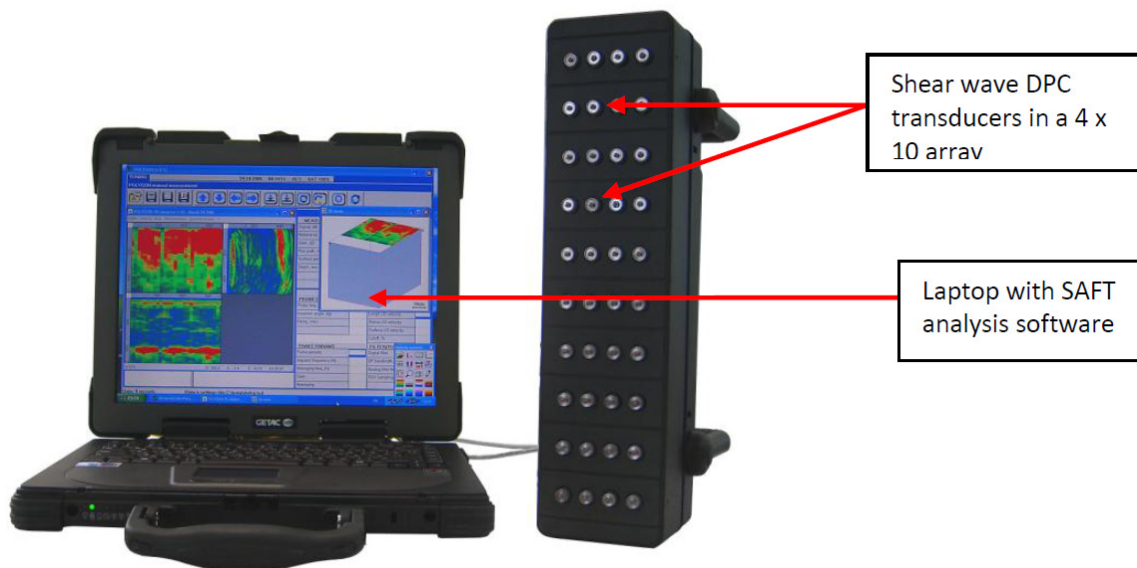
Figure 4: View of the shear wave ultrasonic tomography MIRA system [9]
