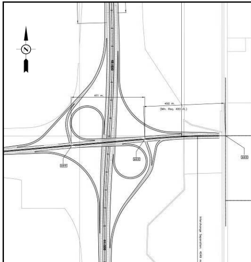
Figure 5 – Modified Parclo A Alternative
