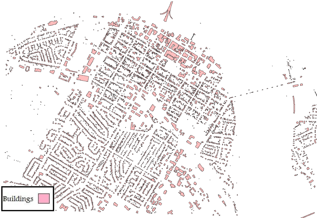
Figure 4: Building footprints extracted using LiDAR point clouds
