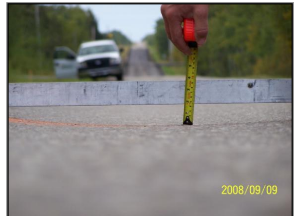
Figure 15 – Measuring Rutting on a Parkland County Road.
