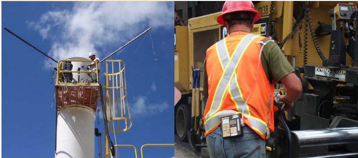
Figure 1: Emissions Measurements Taken at the Asphalt Plant and Asphalt Paver
