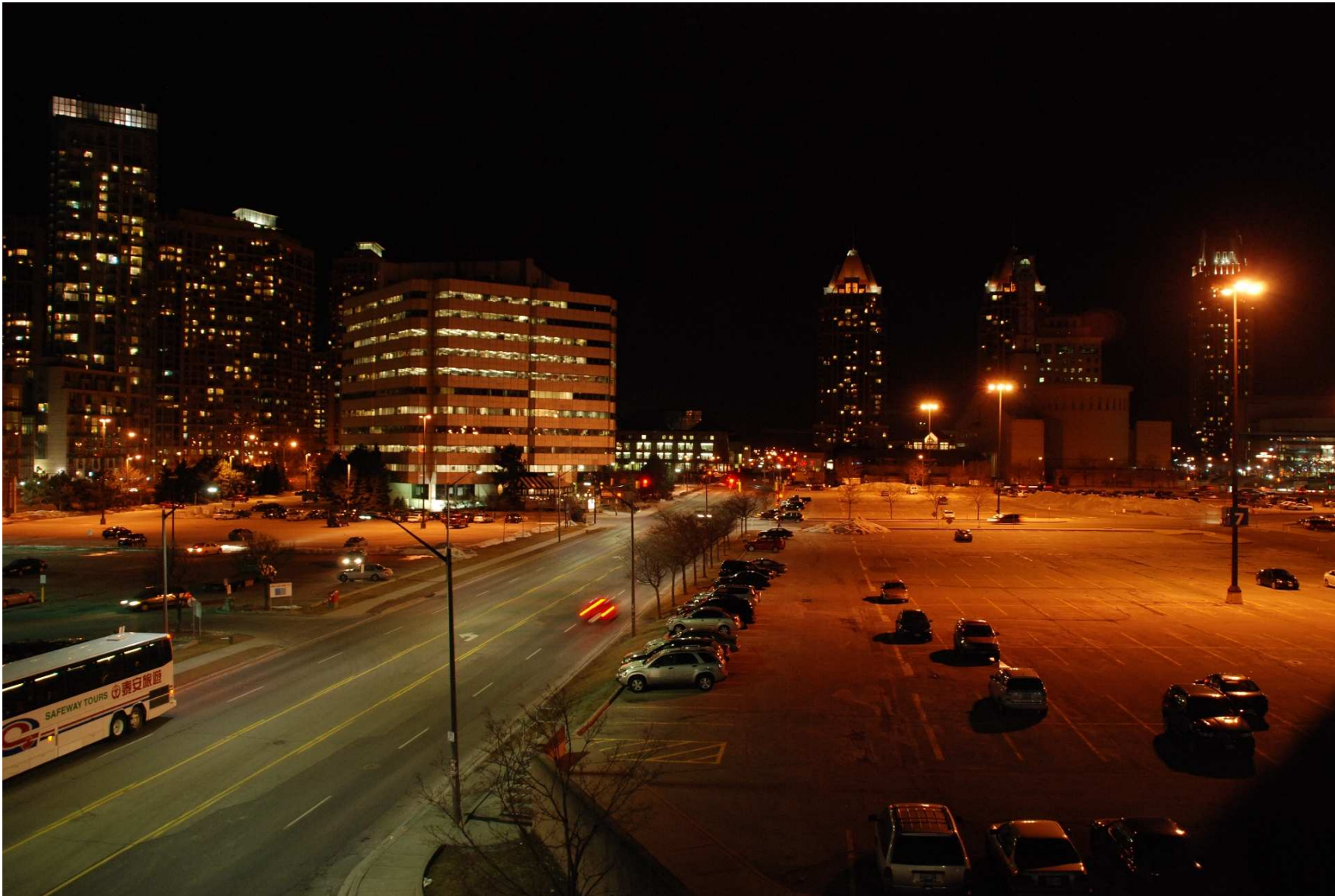
Image 7 - LED Street lights – LED street lights (Left) provide a more uniform distribution of white light, compared to the yellow-orange hue produced by traditional HPS lighting
