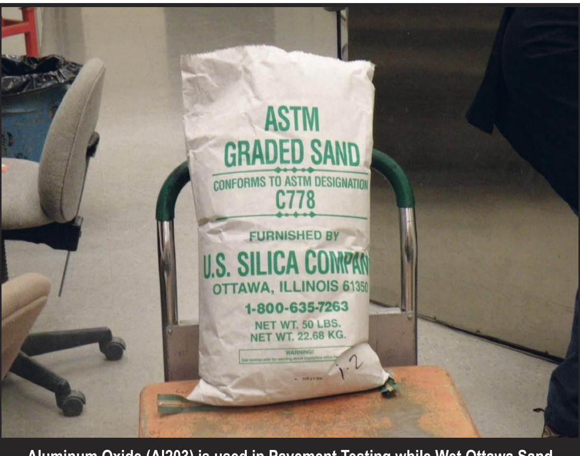
Aluminum Oxide (Al203) is used in Pavement Testing while Wet Ottawa Sand Provides a Test that is more Representative of Culvert Abrasion
