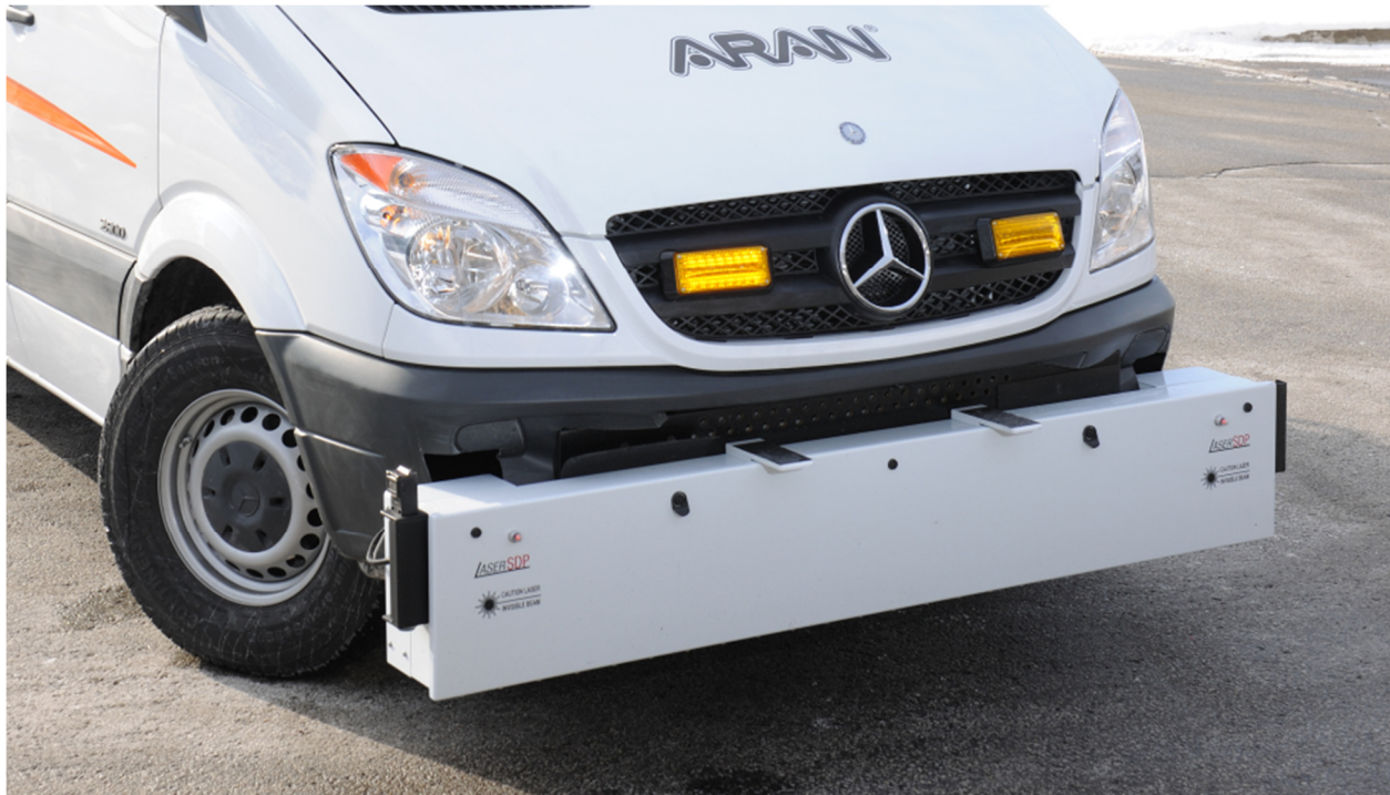
Figure 1. Inertial Profile Enclosure Mounted on an Automatic Road Analyzer
