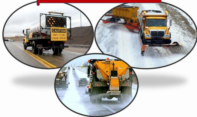
WRM uses large amount of road salt which has become a public concern due to their detrimental effects on environment, infrastructure, and vehicles. Real-time information from road weather information system (RWIS) can help improve the effectiveness of WRM and reduce the salt usage.
