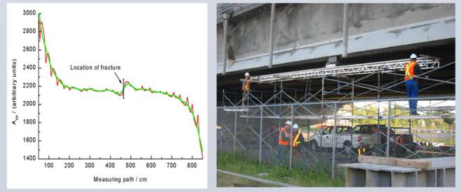
Conduct Remnant Magnetism testing to identify strand/wire fractures or breaks
