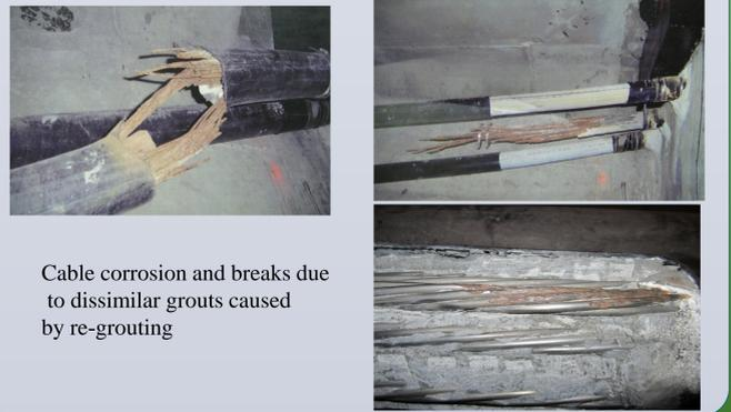
Cable corrosion and breaks due to dissimilar grouts caused by re-grouting
