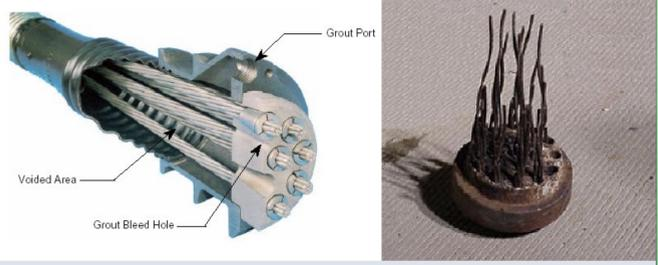
Corrosion of Tendon at Anchor (2000) from Florida Department of Transportation. Most tendon corrosion is within anchorage zone
