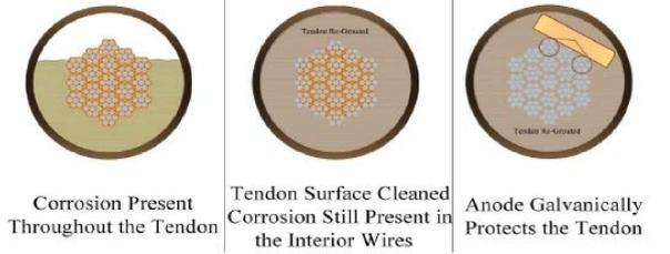
Corrosion Present Throughout the Tendon      Tendon Surface Cleaned Corrosion Still Present in the Interior Wires      Anode Galvanically Protects the Tendon
