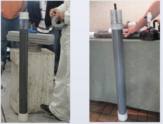
Wick-induced bleed test by American Segmental Bridge Institute in April 2012 showing portland cement grout with about 4% bleeding after 24 hours of grouting operation.
