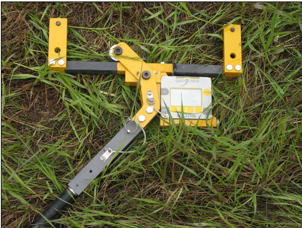
PHOTO 10. Clip on Quick Check Tension Meter (DILLON) to measure tension in the cable.
