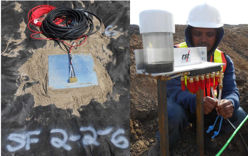
Figure 6. Left: picture of a settlement plate installation and Right: picture of a reservoir for settlement plates in one section.
