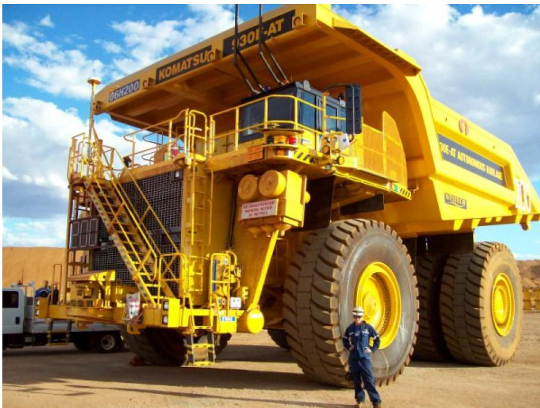
**Figure 1 A Komatsu 930E Using the Frontrunner Autonomous Haulage System technology**
