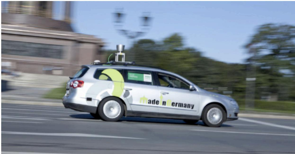
**Figure 3 The AutoNOMOS Labs 'MadelnGermany' autonome**
