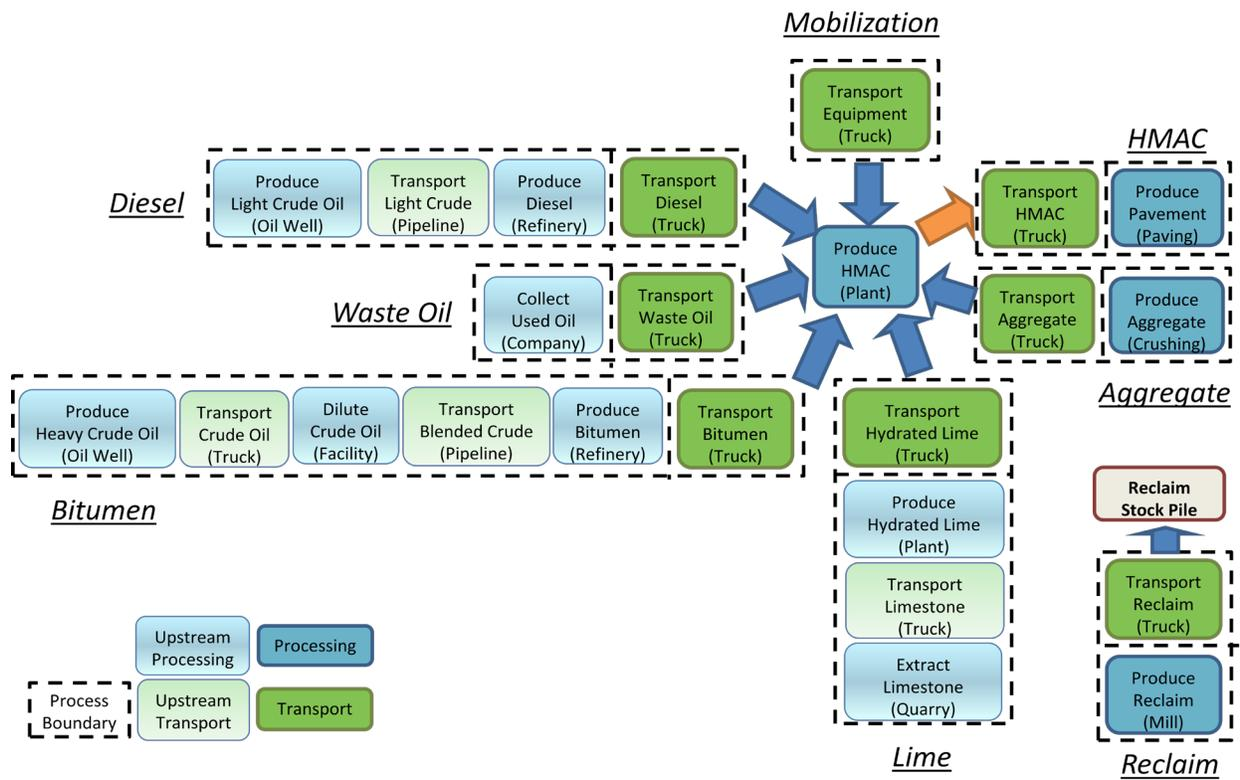
Figure 3. Process flow diagram for conventional AC component of HMAC rehabilitation alternative.
