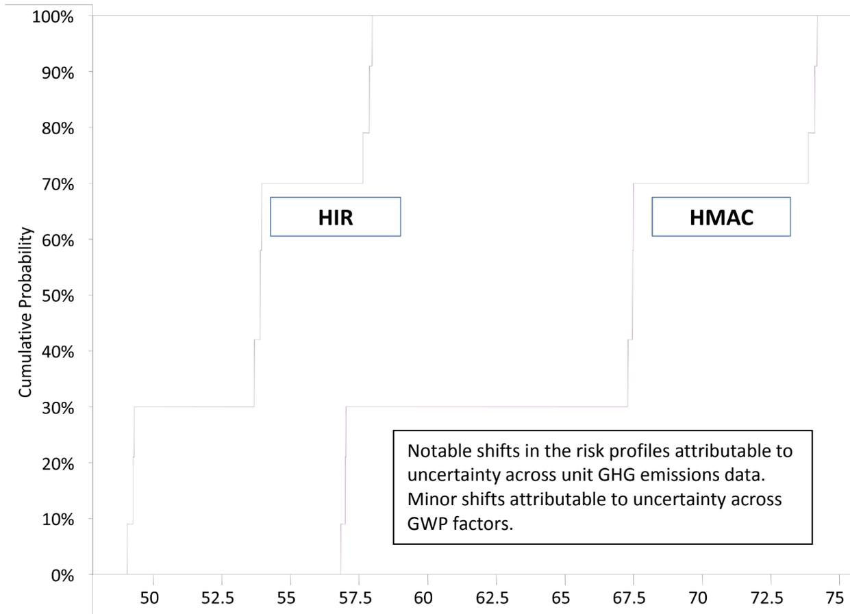
**Figure 4.** Risk profiles of carbon output results (in kg CO<sub>2</sub>e / tonne AC).
