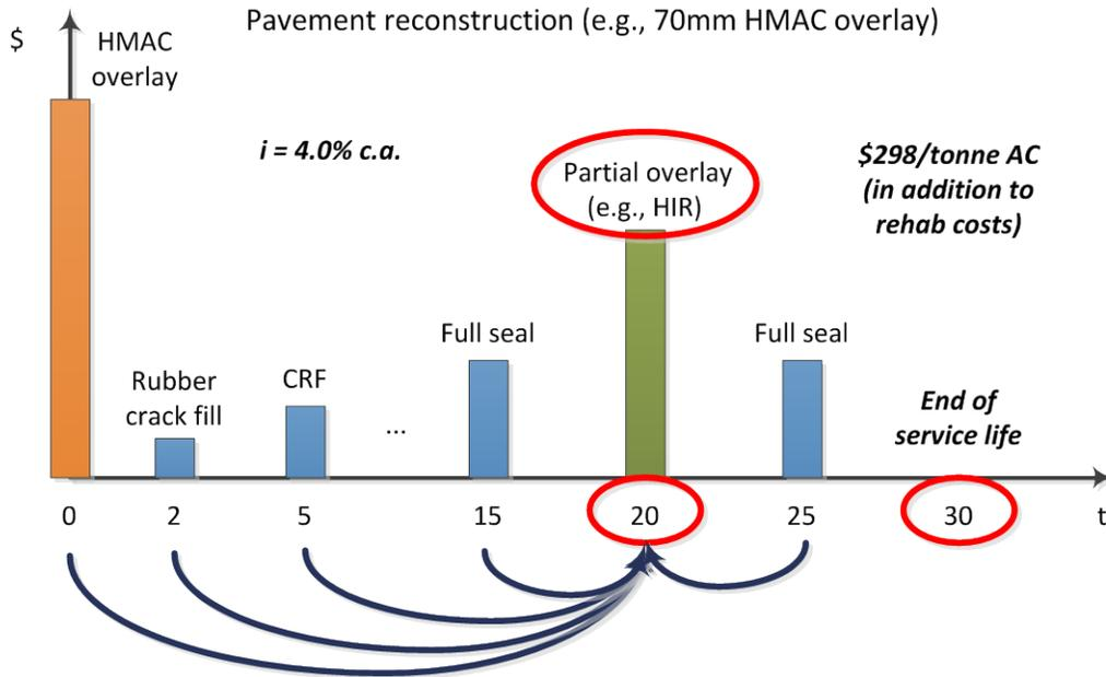
Figure 2. Method of estimating Life Cycle Costs for base Year 20.
