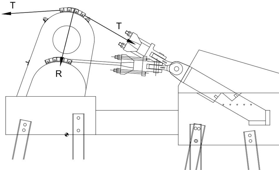
Figure 6: Tower Block resultant force
