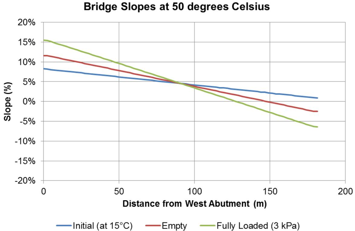
Figure 4: Bridge slopes over the length at 50°C
