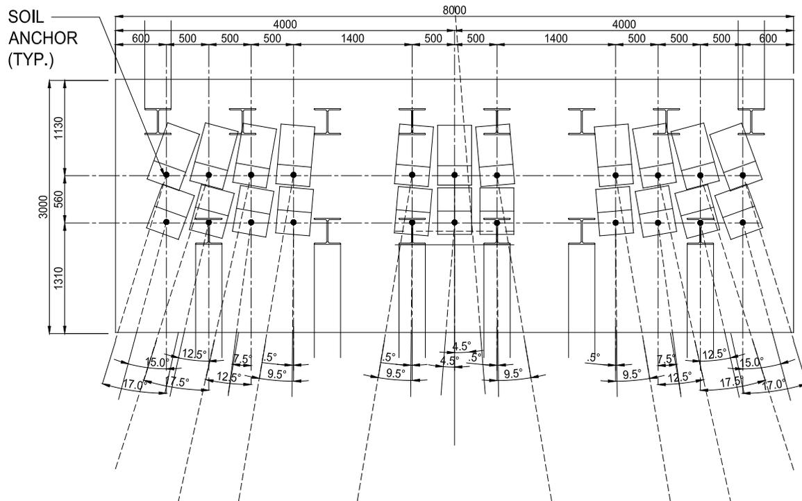
Figure 7: Layout of soil anchors and piles in the anchor block
