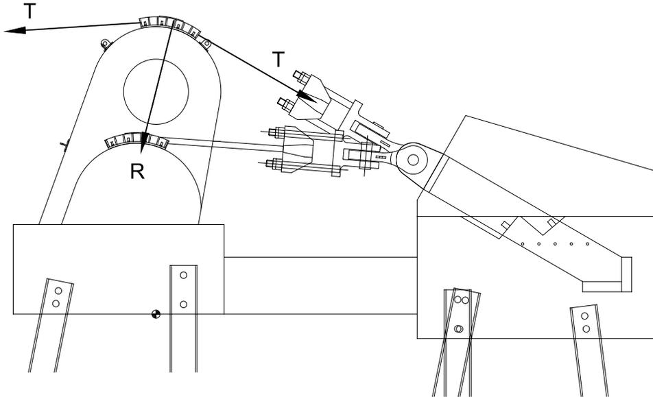
Figure 6: Tower Block resultant force
