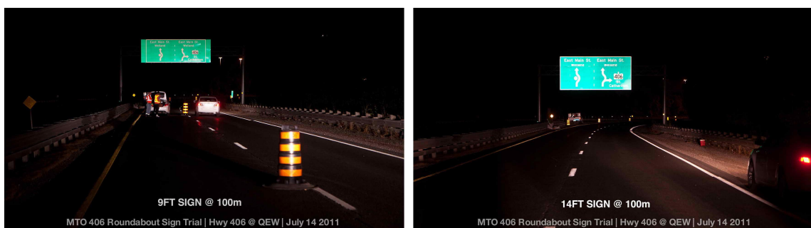
Figure 3.8 Comparison of Overhead Signs. Both signs are shown from a distance of 100 metres.
