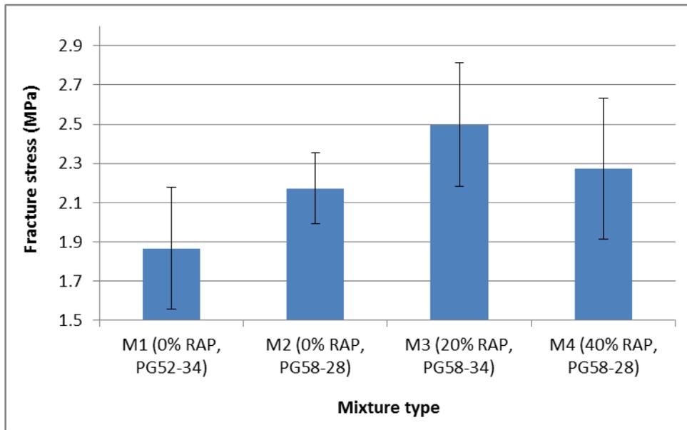
**Figure 4: Fracture Stress of Different Asphalt Concrete Mixtures**
