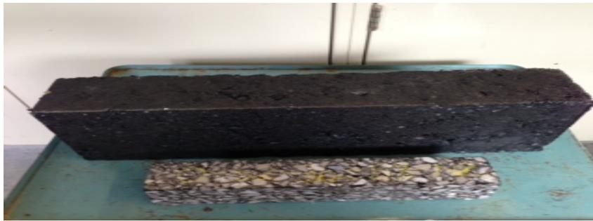
**Figure 1: Compacted Asphalt Beam and Saw-cut TSRST Beam Specimen**
