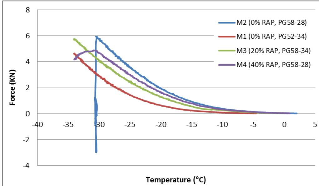
**Figure 3: Typical Force-Temperature Fracture Curves of Tested HMA Mixtures**
