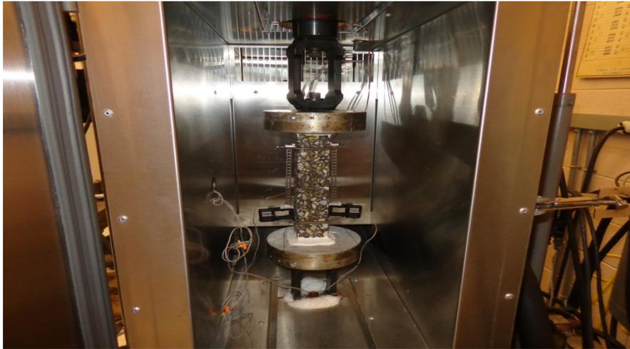
**Figure 2: Typical TSRST Test Setup**
