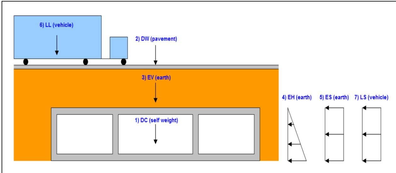
Figure 8 - Design Loads on Concrete Box Culverts
