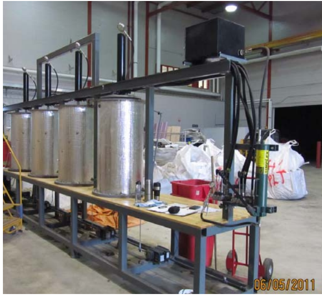
Figure 7 Photograph of compression apparatus for Testing TDA
