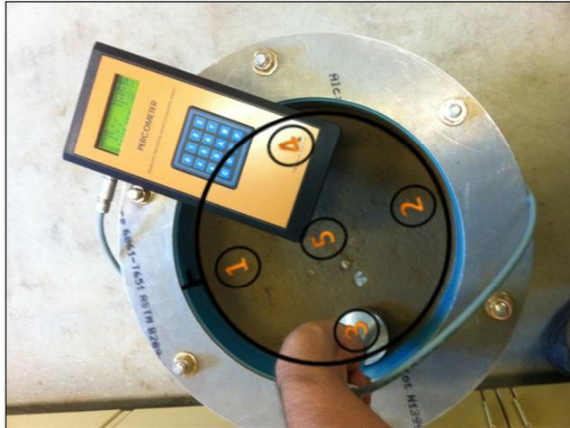
Figure 4. DV measurement at 5 points on the compacted sample surface using a percometer
