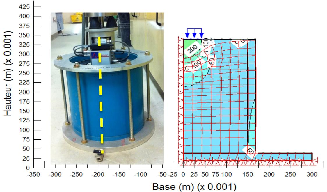
**Figure 3. Simplified test procedure using PLWD for resilient modulus estimation**
