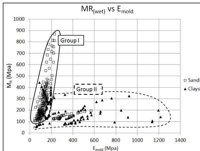
Figure 5. Relationship between  $M_r(\text{wet})$  and  $E_{\text{mold}}$  [6]
