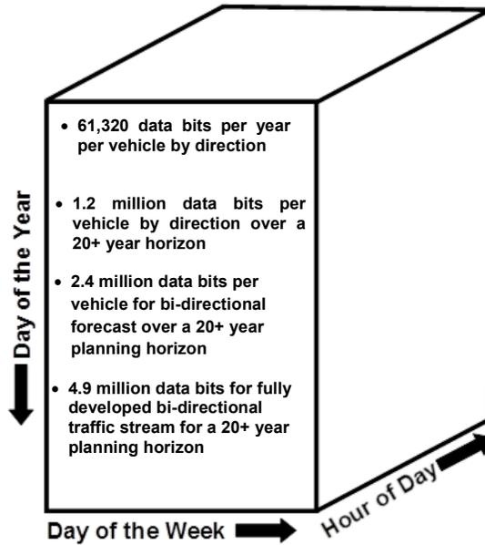
Figure 6: Three Dimensional Relationship Structure of expansion factors for Permanent Counting Stations
