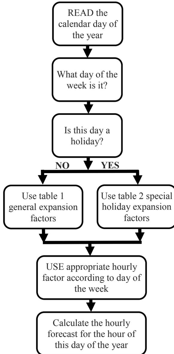
Figure 7: Decision Flowchart for Algorithm Used to Generate Vehicle Forecasts at Pembina-Emerson POE
