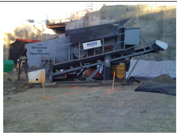
Photo 6 (L) Groundwater treatment process; Photo 7 (R) Soil screening process at Westbrook
