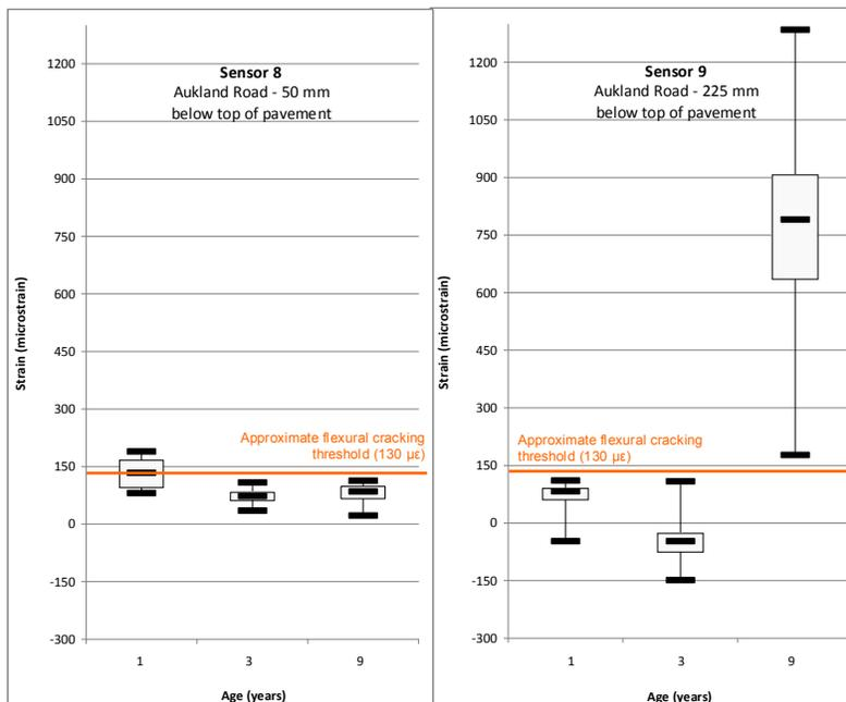
**FIGURE 7 Comparison of strains in JPCP after 1, 3 and 9 years of service.**
