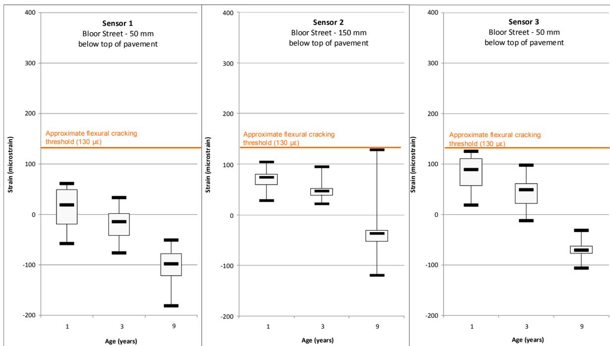
**FIGURE 5 Comparison of strains in unbonded overlay after 1, 3 and 9 years of service.**
