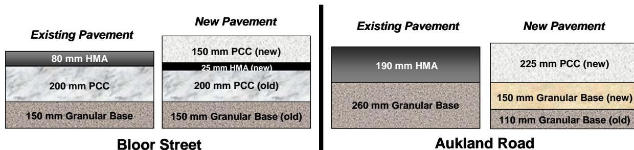
FIGURE 2 Existing and new pavement designs.
