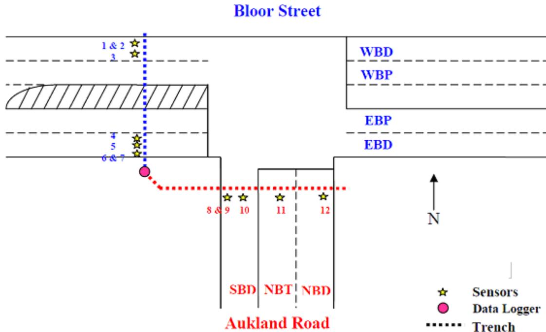
**FIGURE 3 Instrumentation layout.**
