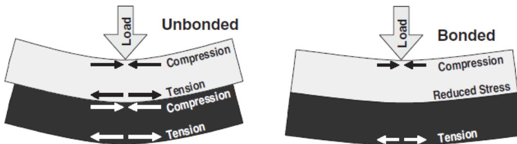
**FIGURE 6 Comparison of unbonded and bonded overlay strain profiles (11)**
