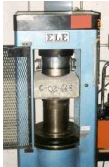
Figure 2 – Test set-up for simulated keyhole testing
