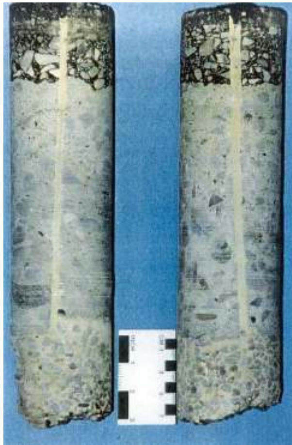
Figure 12 – View of satellite cores taken one month after installation
