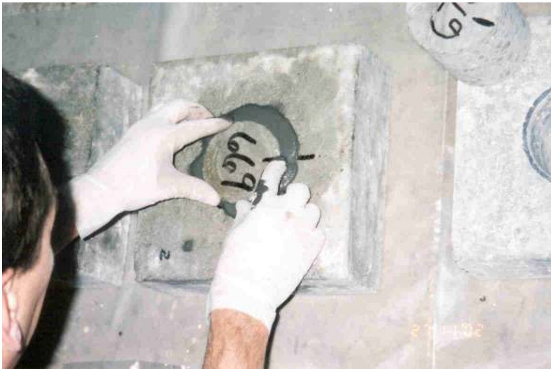
Figure 4 – Core sample being re-instated into slab for push-out testing
