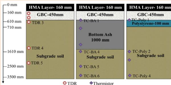
Figure 2- Cross section and as-built depth of thermistors and moisture probes.
