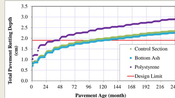
Figure 6- MEPDG-predicted total pavement rutting
