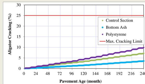
Figure 7- MEPDG-predicted total pavement alligator cracking.
