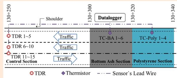
Figure 1- Plan view of the test sections.
