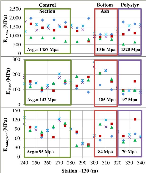
Figure 4- Backcalculated modulus of different layers using EVERCALC
