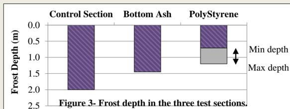
Figure 3- Frost depth in the three test sections.
