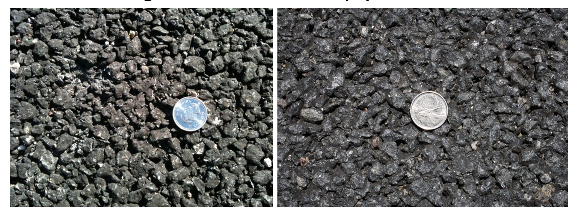
FIGURE 10 – Change in OGFC & OBC Section (A) Surface Macro-texture
