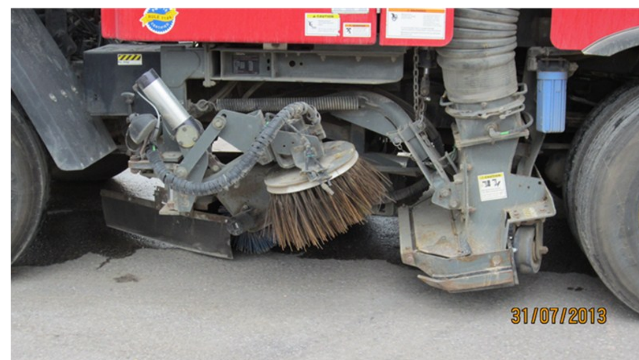
FIGURE 4 – Vacuum Sweeper used to Improve Noise Reduction of Quiet Pavement Sections
