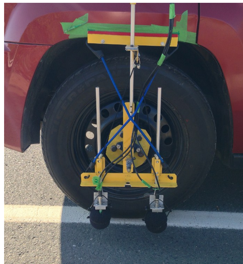
FIGURE 2 – OBSI Microphone Setup
