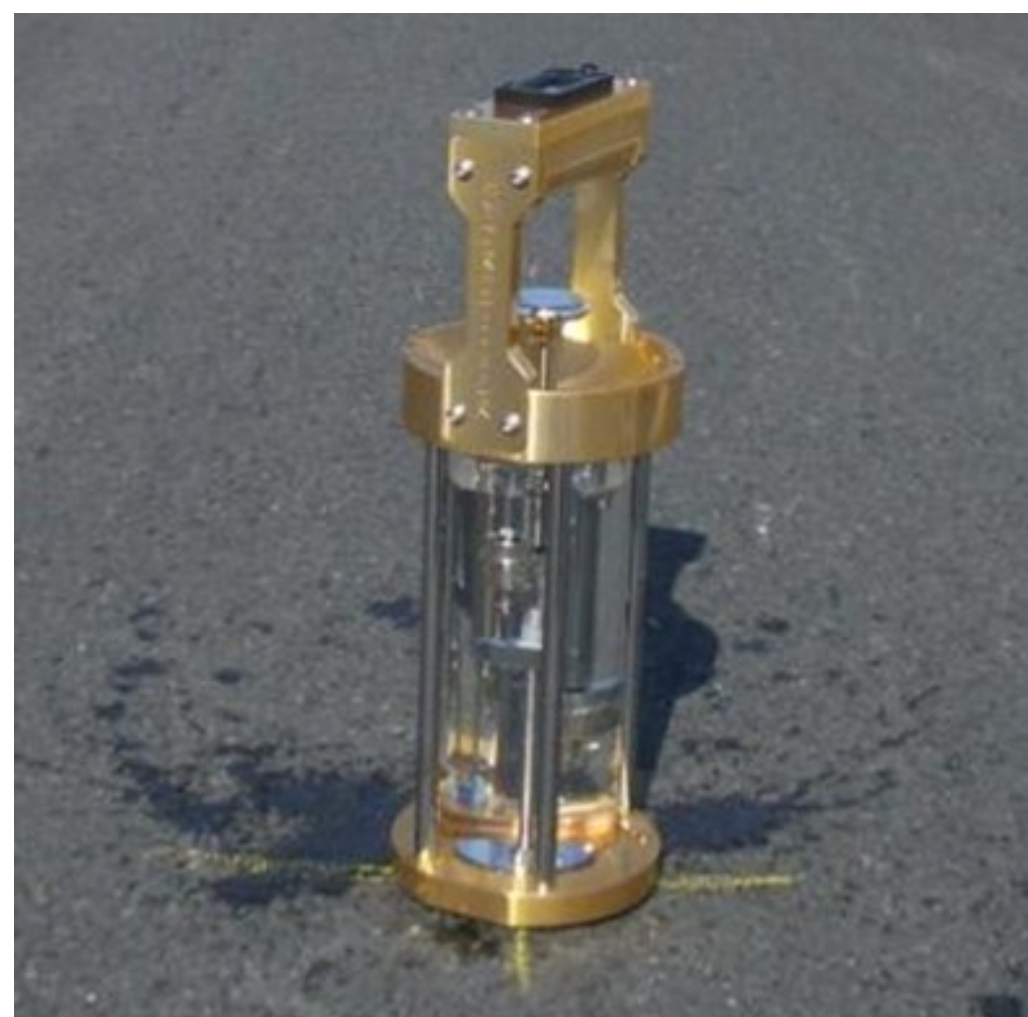
FIGURE 3 – Outflow Meter used to Measure Porosity
