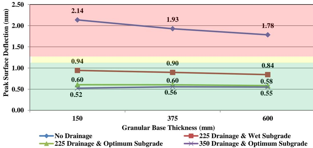
Figure 6 Local Roadway Comparisons (45 mm AC, Type CH Subgrade)
