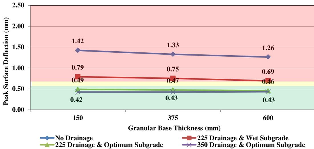
**Figure 8 Arterial Roadway Comparisons (110mm AC, Type CH Subgrade)**
