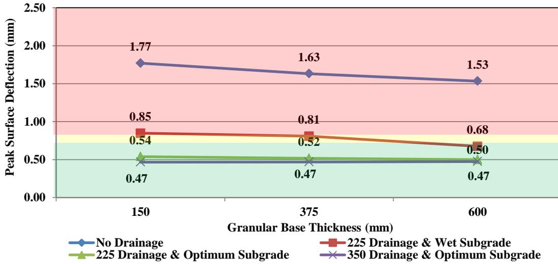
Figure 7 Collector Roadway Comparisons (80mm AC, Type CH Subgrade)
