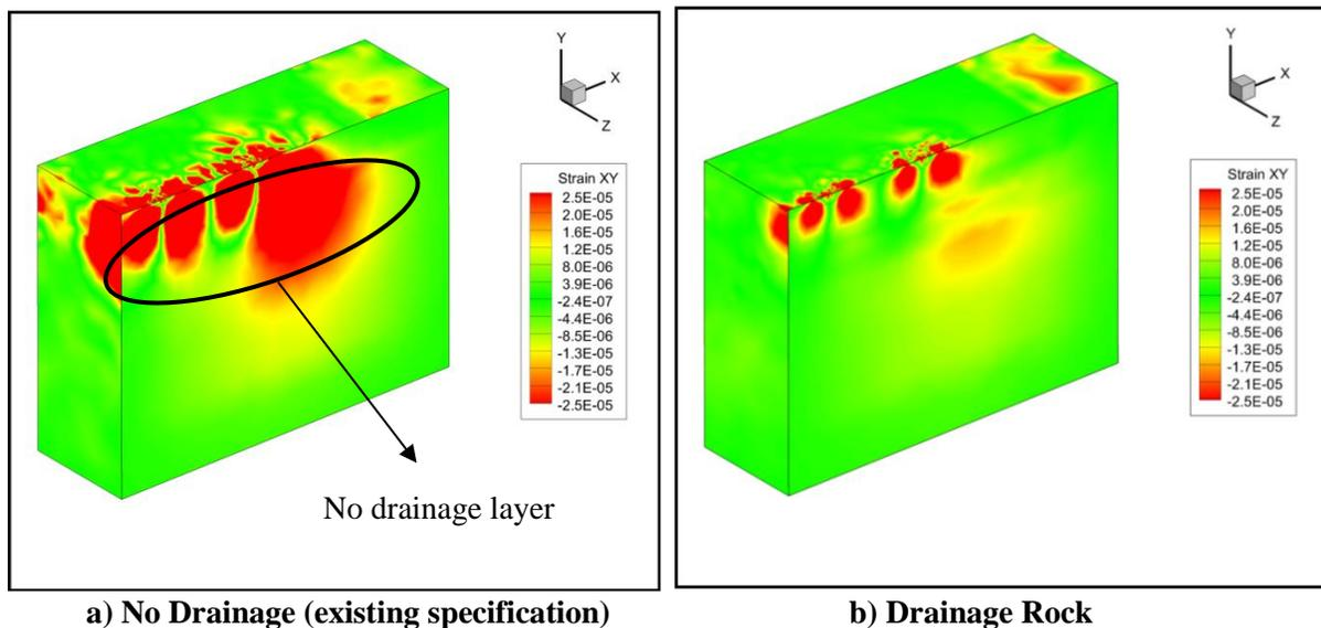
**Figure 3 3D Shear Strain Results – Local Roadways, (CH Subgrade, High Risk of Moisture)**
