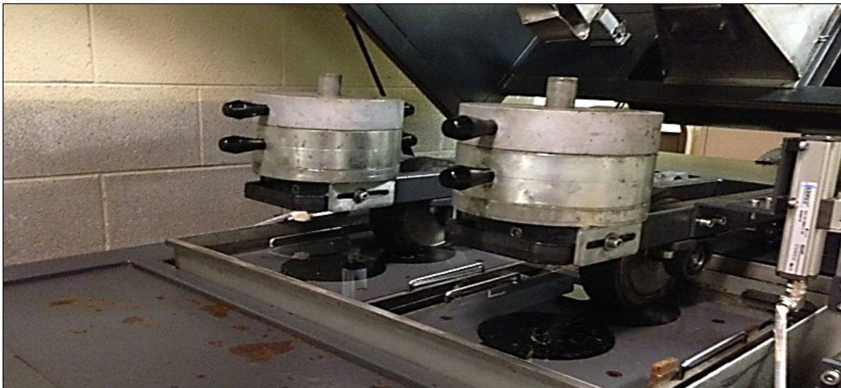
Figure 3: CPATT's Hamburg Wheel Tracking Device (HWTD) Setup
