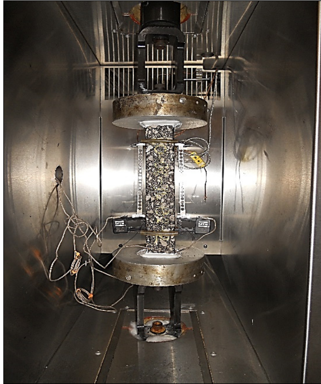
Figure 5: CPATT's Thermal Stress Restrained Specimen Test (TSRST) Setup
