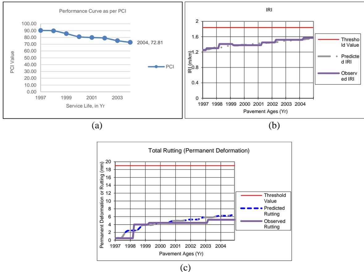
Figure 1: (a) Performance Curve of Base Case as per PCI; (b) Comparison of Observed IRI to Predicted IRI; (c) Comparison of Observed to Predicted Permanent Deformation
