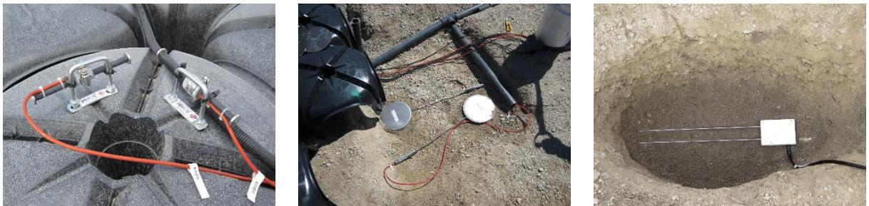
**FIGURE 8 Instrumentation installed in the trial pavement sections.**
