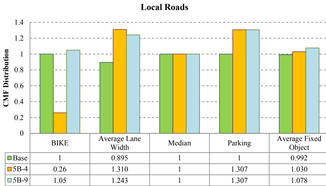
Figure 2: Comparison of Base Condition and the Lowest (5B-4) and Highest (5B-9) Safety Risk Cross Sections Based on CMF Distribution for Local Roads
