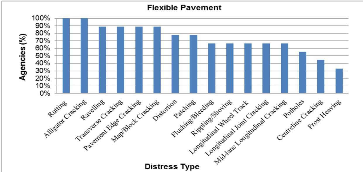
**Figure 2: Percentage of Agencies Collecting Flexible Pavement distresses**
