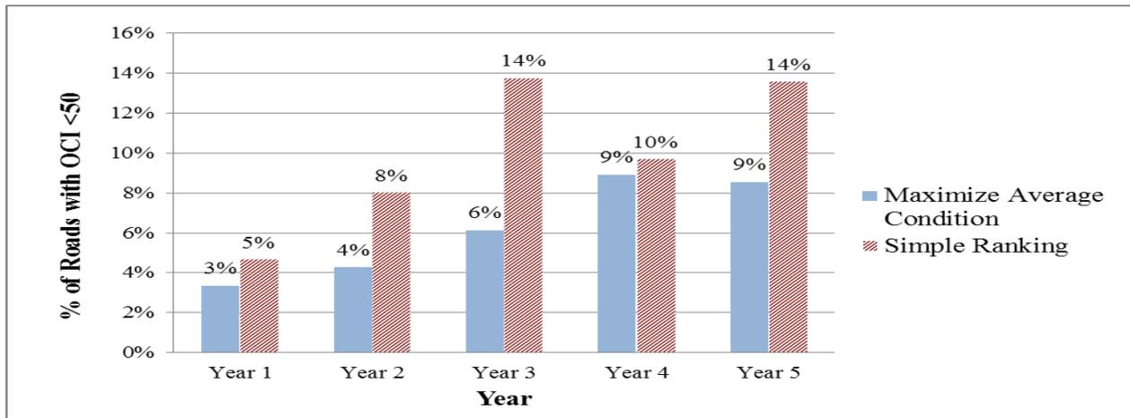
**Figure 7: Percentage of Roads with OCI < 50 Using Simple Ranking and Evolver**
