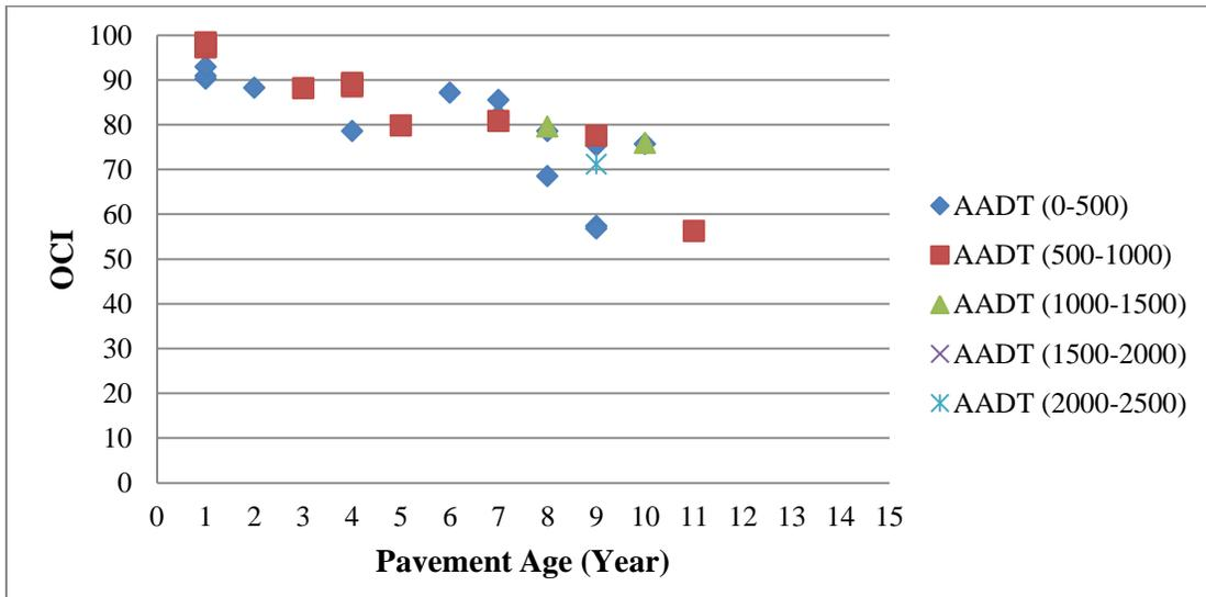
**Figure 0: Local Roads with Shave and Pave Treatment for Different AADT**
