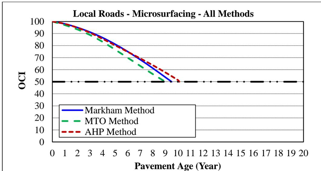
Figure 6: Pavement Performance Prediction Model for Local Roads with the Microsurfacing Treatment
