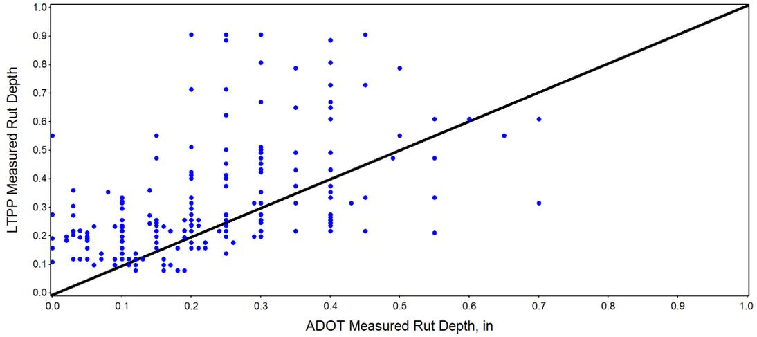
Figure 3. Relationship between ADOT and LTPP Rutting Measurements.
