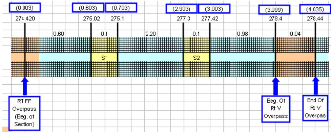
Figure 8. Illustration of a typical MoDOT project and 500-ft sample units.
