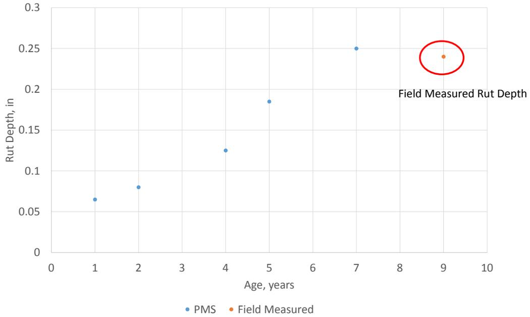
Figure 5. Relationship between field measured and CDOT PMS rut depth measurements for PMS Project 10-12393.
