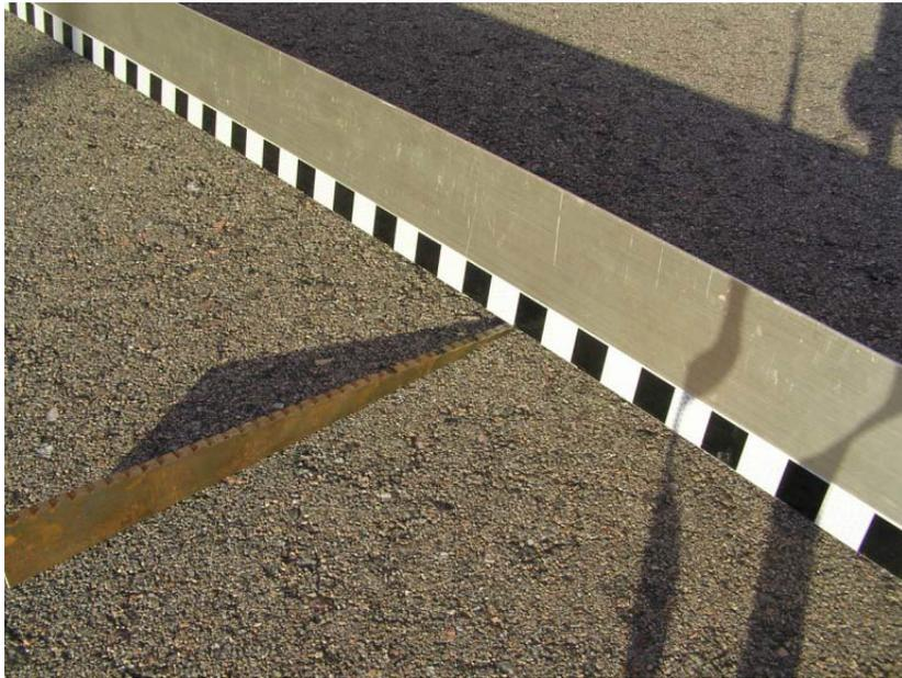
Figure 2. Straight edge method for measuring rut depth.
