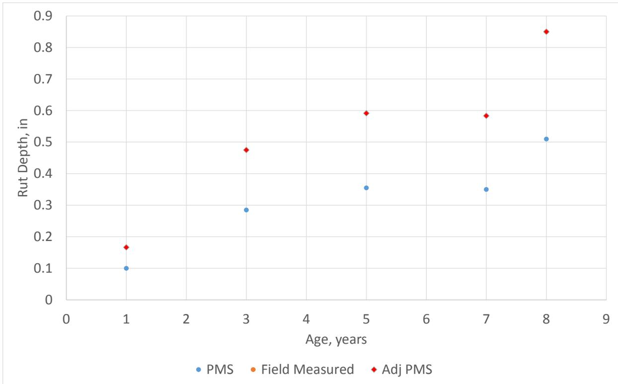
Figure 7. Plot showing adjusted and CDOT PMS rut depth measurements for PMS Project 27-13959.
