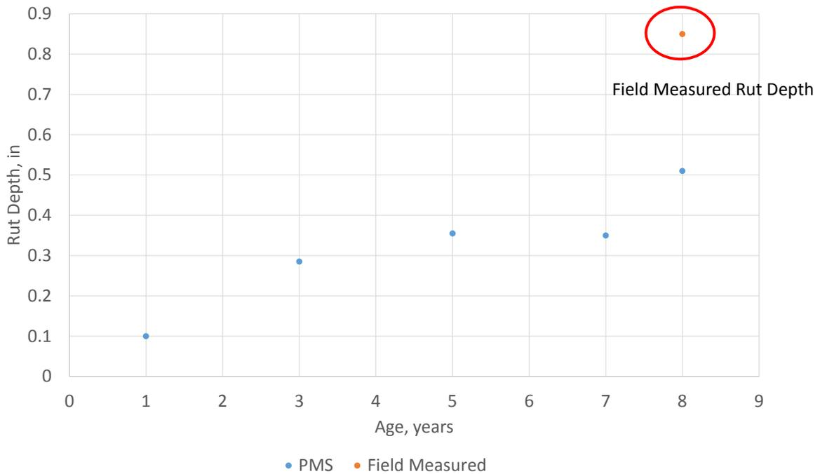
Figure 6. Relationship between field measured and CDOT PMS rut depth measurements for PMS Project 27-13959.
