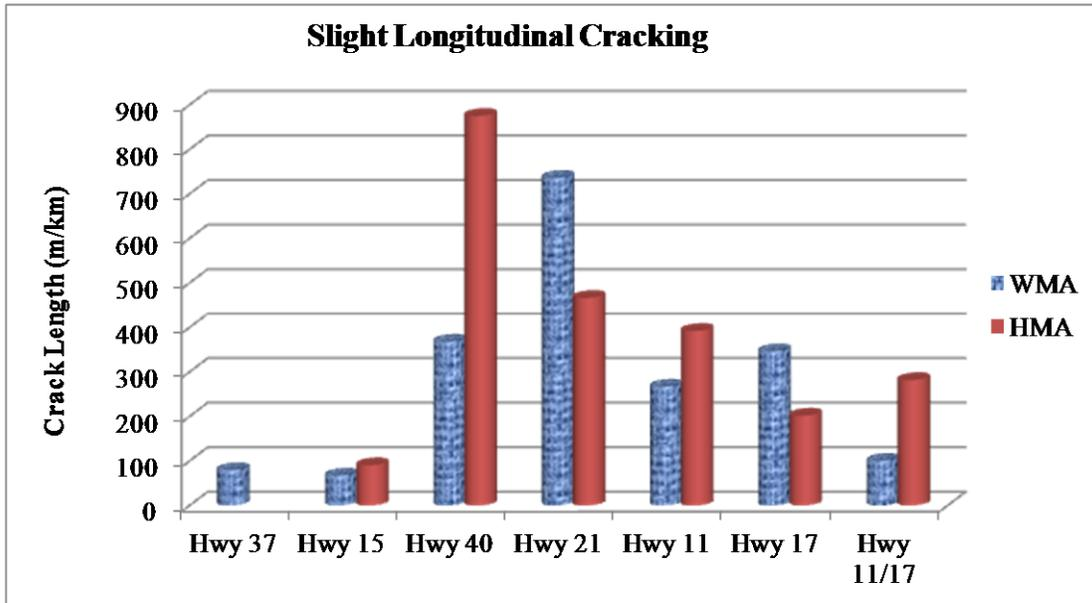
Figure 11 – Extent of slight severity longitudinal cracking on the WMA and HMA sections
