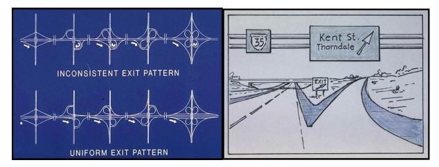
Figure 12 – Single exit, on right, advance of crossroad, simplified signing
