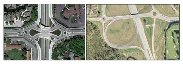
Figure 14 – Interchanges with Roundabouts
