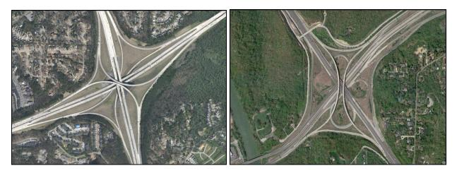
Figure 9 – All Directional Interchange and Directional with Two Loop Ramps
