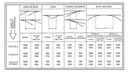
Figure 13 – Jack Leisch Original Table (1975) for Ramp Spacing Guidelines
