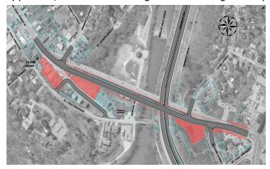
substandard sightlines and approach curve. However, it considerable would require property acquisition implement. The connection at north approach would require the introduction of back to back horizontal curves, a less desirable aeometric solution. Additionally, the north approach alignment would impact existing public lands which contain graves.
