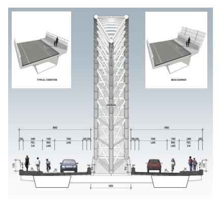
delved deeply into the heritage features of the project location for the inspiration to create an environmentally responsible structure with landmark and iconic characteristics. Only a few bridges around the world comprise the forebears of the new Burgoyne Bridge, which is a multi-span structural steel box girder bridge with a long span steel arch that includes elements of the old cable-stayed swing bridge which once crossed the river at this site.
