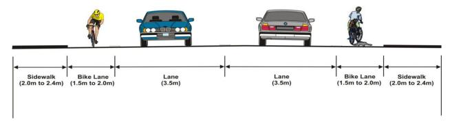
As the approach roads are only two lanes wide, the bridge structure included two travel lanes with bike lanes and sidewalk on either side, however in the future, should the approach roads require widening to four lanes, the bridge could be
