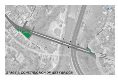
Stage 2 – Divert traffic to the east portion of the new bridge and remove existing bridge. Construct west portion of the bridge.
