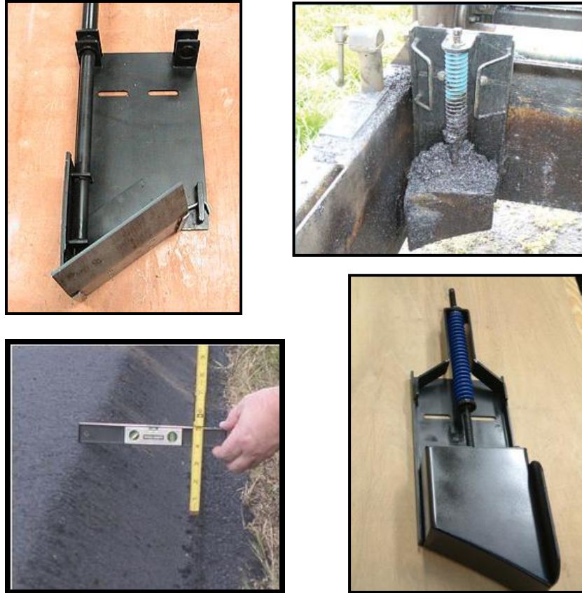
Figure 2: FHWA approved 'Safety Edge' sample devices (Picture credit to FHWA and Carlson Paving)
