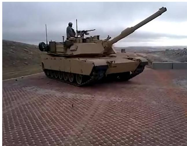
**Figure 3. Permeable pavement to accommodate tanks**
