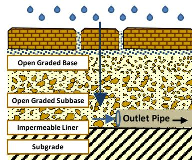
**Figure 2c. No Infiltration**
