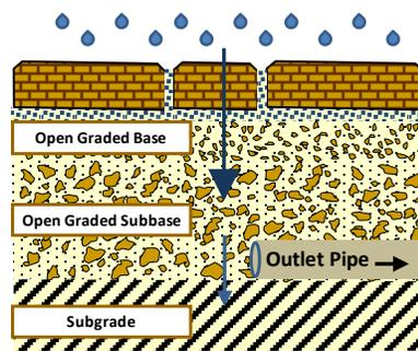
**Figure 2b. Partial Infiltration**
