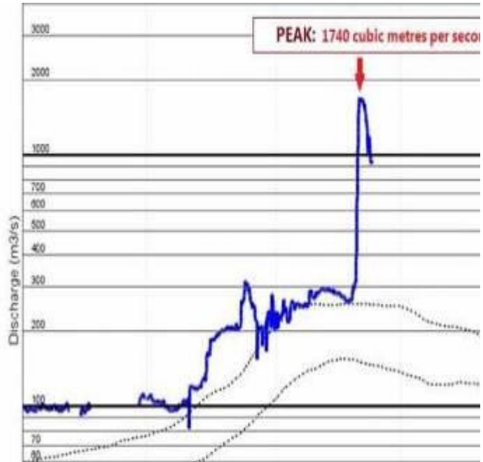
Figure 2: Hourly Increase in Water Level Through Bow River During Flood
