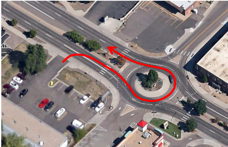
Figure 2.1 Left Turn From Right-Turns-Only Driveway Using Roundabout
