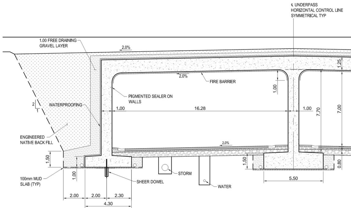
FIGURE 4 – TYPICAL SECTION OF TUNNEL WITHOUT APPROACH SLAB, AREAS AWAY FROM TAXIWAYS AND RUNWAY
