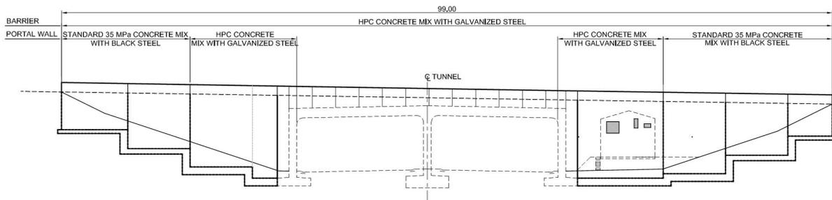
FIGURE 5 – ELEVATION OF TUNNEL PORTAL, SHOWING STEPPED FOOTINGS AND CONTROL BUILDING
