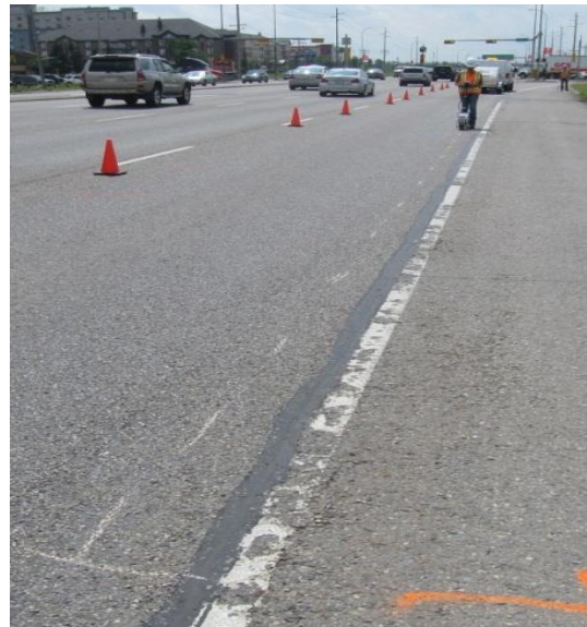
Figure 2: Example of 25 m Line Being Measured Using the SurPRO
