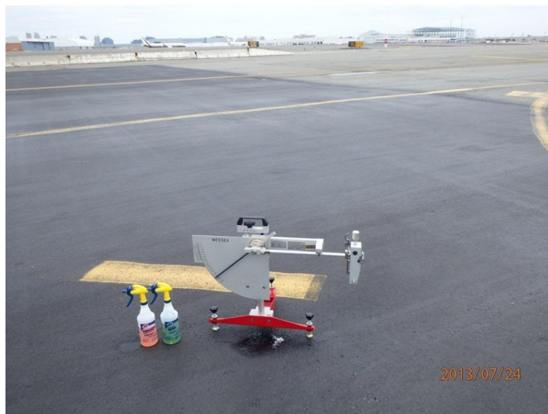
Figure 8: BPT Equipment on Sealed Asphalt Pavement
