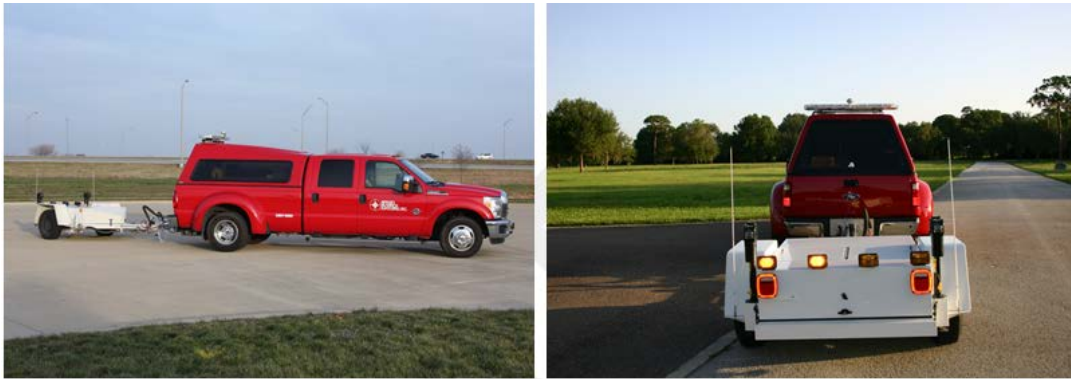
Figure 3. Vehicle and Testing Trailer Used to Complete the Skid Testing
