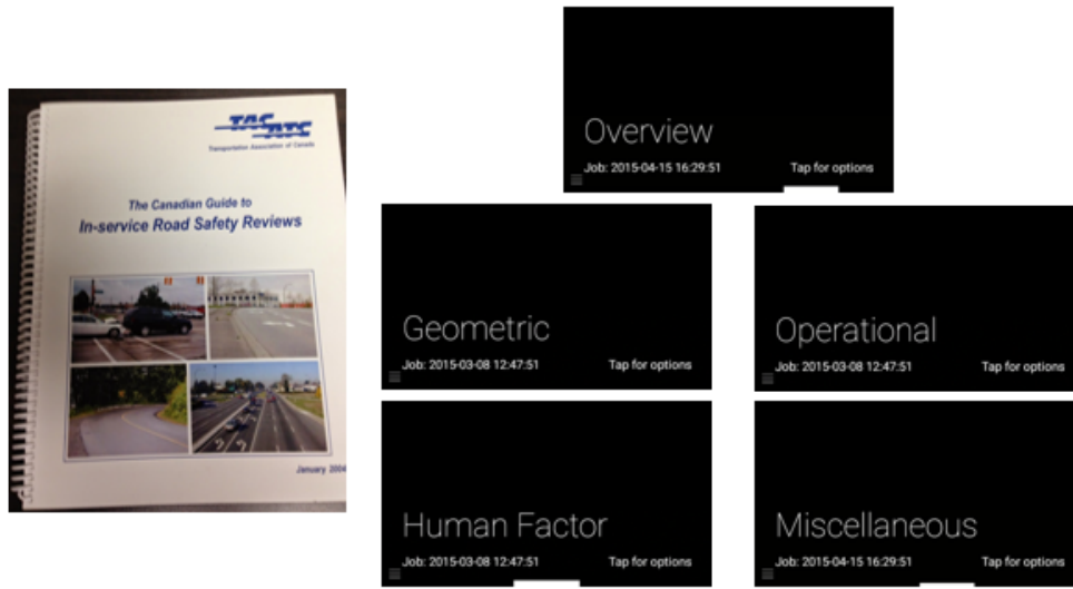
Figure 7: Application records issues and treatments in five categories based on the TAC Guide (viewed on prism screen on glass, activated by touch or voice input)
