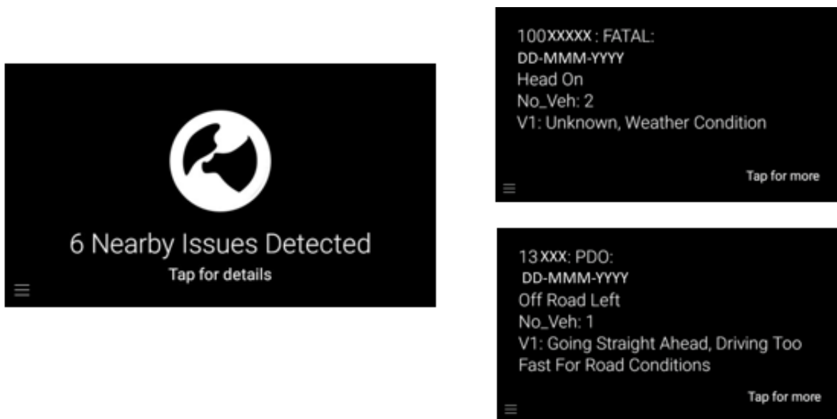
Figure 10: Applications provides user with 'pop-up' geo-referenced contextual notifications of collision information. It can also provide any other location based information such as site details or citizen concerns linked to the site. (viewed on prism screen on glass)
